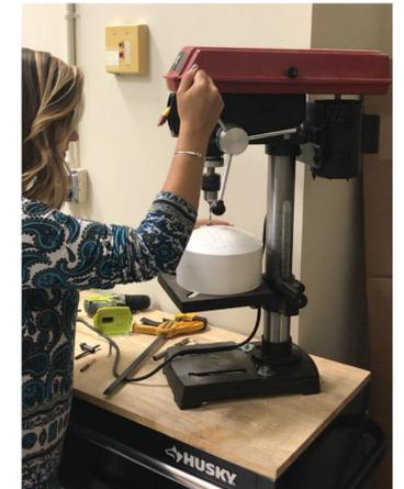
The PVC frame has a simple construction process. This involves cutting a PVC pipe into 4" and 6" sections, and drilling holes into the PVC endcap for water to pass through.
